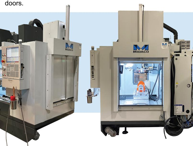
**MIDACO Industrial Robot Access Doors** provide just the right solution for machine shops that require a specialized production set-up with unconventional access to their machine tools. MIDACO can design and install a pneumatic access door on CNC machining centers, VTL's, grinders and virtually any enclosed machine.
