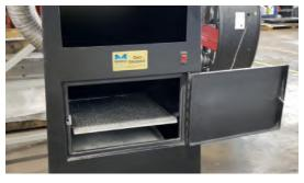
The easily replaced or cleaned collection filter is made up of 3 grades of treated, flame retardant filter material to offer maximum performance and reduction in the amount of dust and grit discharged into the work area. An aluminum mesh screen "spark arrestor" is included and sits on top of the filter.
