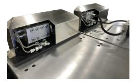
When new parts are put onto the pallet, the Hydraulic Docking System locks fixtures or vices into place and the pallet enters the machining center WITHOUT HOSES.
