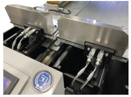
Clamping fixtures or vices will **STAY CHARGED** on the pallet **WITHOUT HOSES** while in the machining center.
