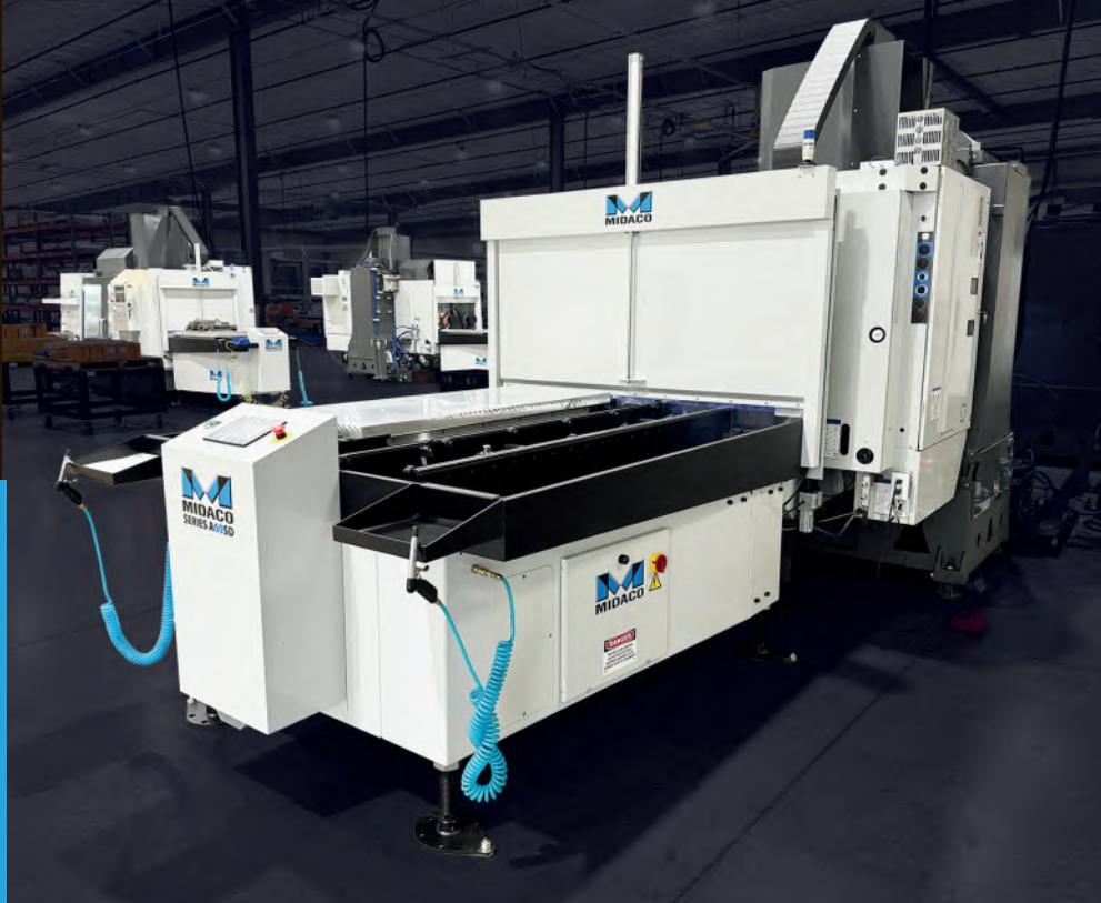
Pallet Changers are one of the most practical and cost-effective ways to boost machining center Overall Equipment Effectiveness (OEE). Many shops associate "automation" with robotics or full FMS setups, overlooking the simpler Automatic Pallet Changer solution.
