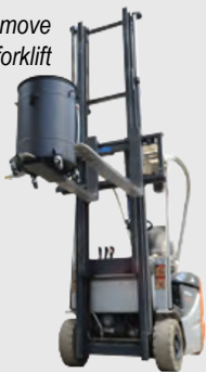
micro-perforated carbon steel basket with added 150 micron PPL filter for very fine chips
