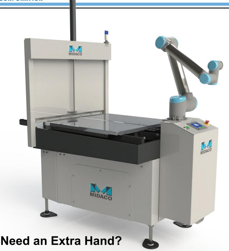
MIDACO's A30SD & A40SD series Automatic Pallet Changers can be modified to mount Robot/Cobot arms directly on the pallet changer control panel for enhanced collaborative automation.
