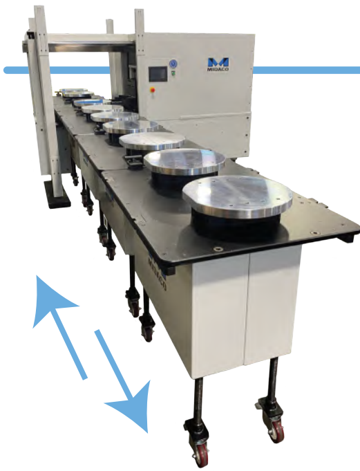
Individual carts are connected via locking T-pins
