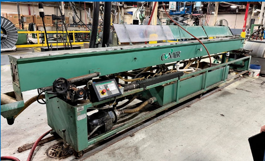
Downstream Equipment Including Vacuum Sizing Tanks, Pullers, Two-Reel Sizing Reels
