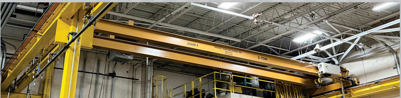
5 Ton x 50' Span Product Handling Design Double-Girder Bridge Crane
